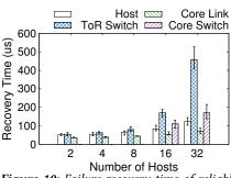
Figure 10: Failure recovery time of reliable 1Pipe. Error bars show  $5^{th}$  and  $95^{th}$  percentile.
