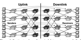
**Figure 3:** Routing topology of a typical data center network. Each physical switch is split into two logical switches, one for uplink and one for downlink. Dashed virtual link between corresponding uplink and downlink switch indicates "loopback" traffic from a lower-layer switch or host to another one.
