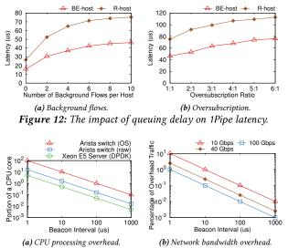
**Figure 13:** Beacon overhead under different beacon intervals. CPU processing overhead for Arista switch is extrapolated.
