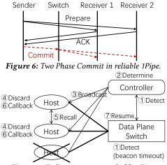
Figure 7: Failure recovery in reliable 1Pipe.
