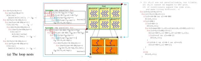
(b) The code and GPU mapping of a conservative fusion heuristic
