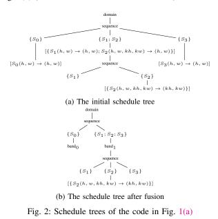
A band node is used to represent a loop nest, and the attached information is used to guide the compiler to apply transformations. The content of the band node  $band_0$  is an
